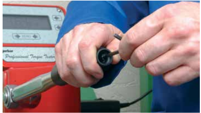
Setting a 'P' Type Torque Wrench
